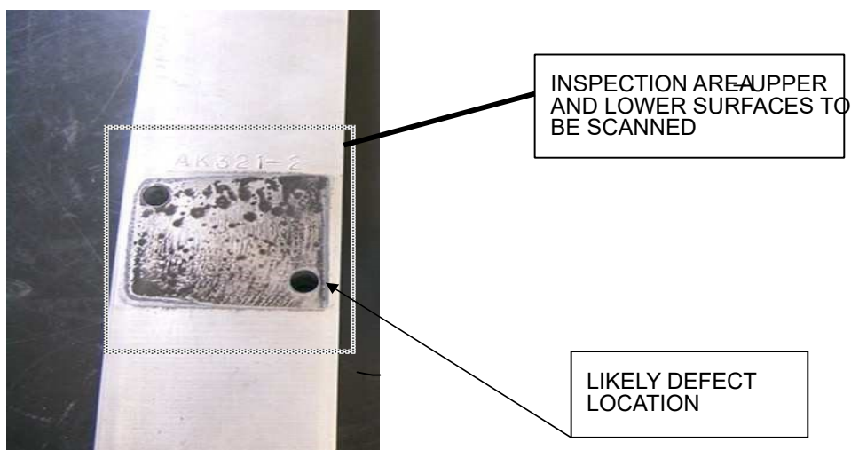
Figure 3: Hub Bar Showing Possible Defect Location and Scan Areas
