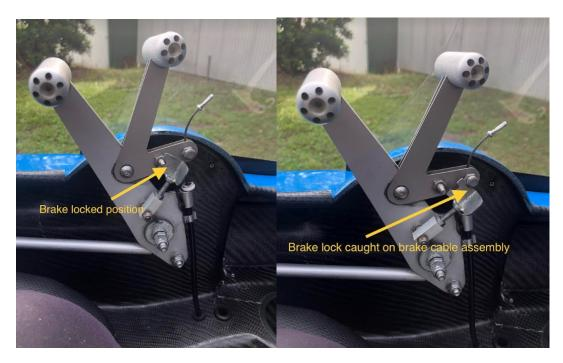
After releasing the park brake, complete a visual check to confirm that the park brake has been completely released prior to take-off. The lock when disengaged will normally pivot downward approximately 90 degrees, but in the accident case it caught on the cable nut keeping the brakes locked.
