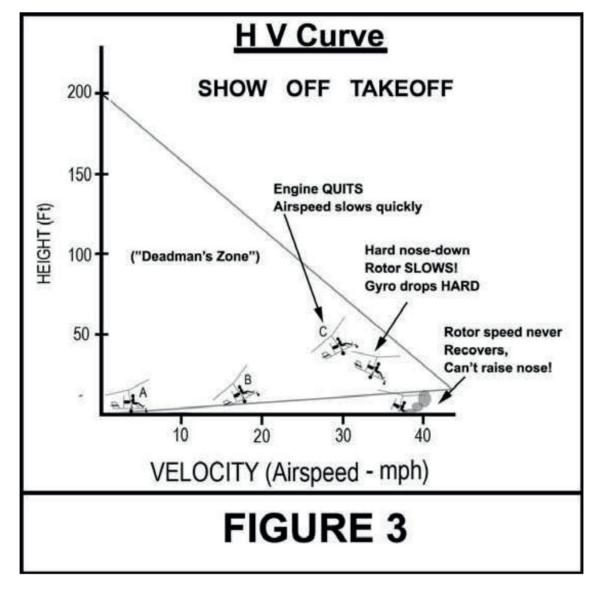
rotor rpm and the subsequent re-loading of the rotor to full airflow and G-Load might not allow quick recovery of the rotor rpm – basically 'over-running' the rotor in flight! In the extreme, the rotor could actually violently 'flap' – hit the teeter stops!
