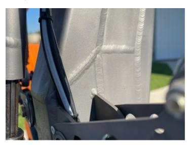
The owner of a Titanium Explorer gyroplane reported finding a cracked weld in the mast of his gyro during a routine pre-flight inspection. An investigation has been carried out by TAG Aviation to determine the cause of this crack. It appears the weld was under stress.
