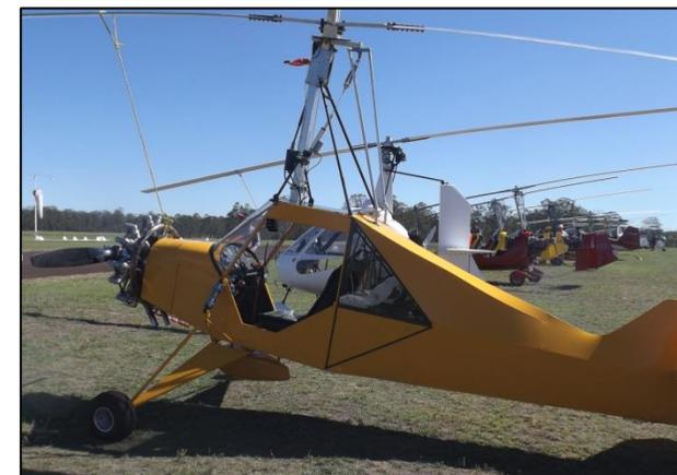
procedure to land after a power failure is the same procedure as a normal landing, which can require no landing roll. Thus the gyroplane is a safer aircraft for low and slow flight, as compared with both helicopters and airplanes. The ability of gyroplanes to fly faster than helicopters and slower than airplanes makes it something of a hybrid, having the good qualities of the other two types of aircraft with little of the bad.
