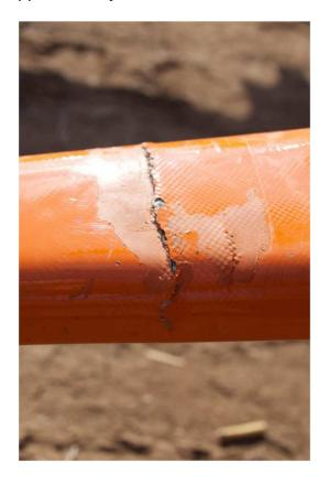
In both cases, the non-slip material was wrapped around the leg such that the cracks were not visible until they had progressed to a point where they were not hidden by the non-slip material.
