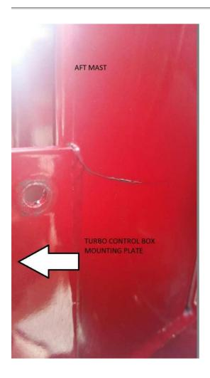
The manufacturer was contacted and advised that there was no suitable repair available and that a new airframe would be required.
